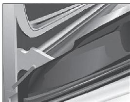
Take hold of the door on both sides. Pull the oven door forward until it is totally free from the hinges (F).
