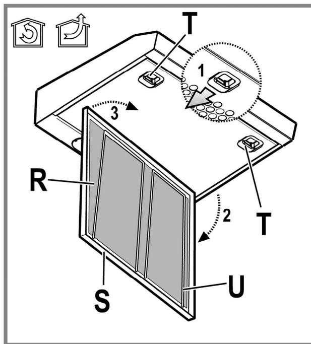
*The self-supporting metal filter* does not include a support grill, in order to remove the filter – pull the release springs backwards and slide the filter downwards.
